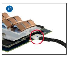
2. Install the SSD into the Mac Pro, as shown below. Insert the SSD at a shallow angle, making sure that the power cable is out of the way.
