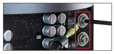
6. Properly installed, the Aura SSD for Mac Pro and power cable will look like the picture below (left). Replace the outer case of the Mac Pro as shown in the picture below (right). When the outer case is seated fully, slide the lock switch back to its original locked position.
