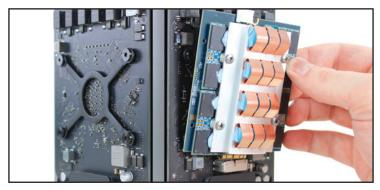
3. Before proceeding, verify that the SSD is fully seated in the connector on the Mac Pro and that the screw hole in the SSD lines up with the screw hole in the Mac Pro. Then, use the included driver and drive mount screw to secure the SSD.
