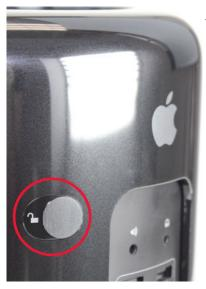
1. Turn off your Mac Pro and unplug all cables, including the power cable. Make sure the lock switch on the outer case is set to the unlocked position (circled at left), then remove the outer case by lifting it straight up. Set aside the outer case and proceed to the next step.
