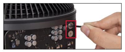
5. First, thread the two included washers onto the two included Torx T8 screws. Next, align the rings on the power cables with the two screw holes, then secure each cable to the power terminals as shown below. Make sure the screws are tightened enough that the power cables cannot rotate in place or move. NOTE: the black wire or black sleeve should always be on the bottom and the yellow portion of the cable should be on the top.
