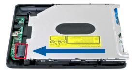
3. Using a Phillips screwdriver, affix three of the collared screws into the screw holes along the side and rear portion of the case, as shown at right.
