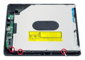
4. Put the top case back on the bottom case and push toward the left, as shown. This will seat the top case into the tabs mentioned in Step 1 and secure the enclosure.
