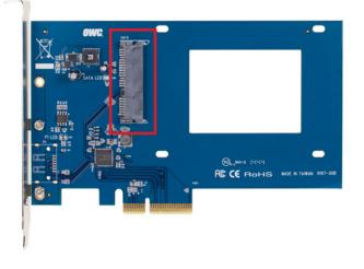
Set the OWC Accelsior S down on a flat surface. Make sure the black SATA connector is facing up, as shown above.
