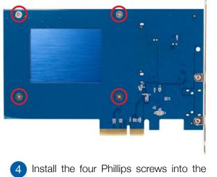
Install the four Phillips screws into the four screw holes to secure the drive to the Accelsior S, as shown.
