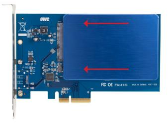
Slide the SATA connector on the drive into the SATA connector on the Accelsior S. Ensure the drive is fully seated, as shown.
