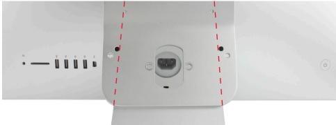
3. Use the clamp to secure the NuMount VESA adapter to the iMac stand. Place the clamp in the hole in the iMac stand with the rubber O-ring on the clamp facing the adapter. Line up the screw holes in the clamp with the screw holes in the adapter and use the included hex key and the longer socket-head screws to fasten the clamp to the adapter. The following set of pictures shows this process from the front, side, and rear respectively.
